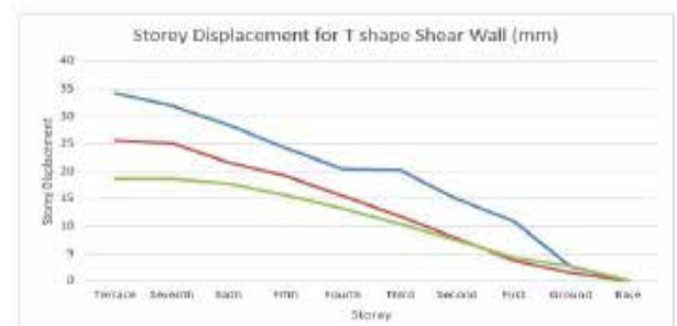
Figure 14:-Graph for Storey Displacement for T shaped shear wall
