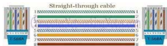
Fig.1 color for lan connection in Straight
