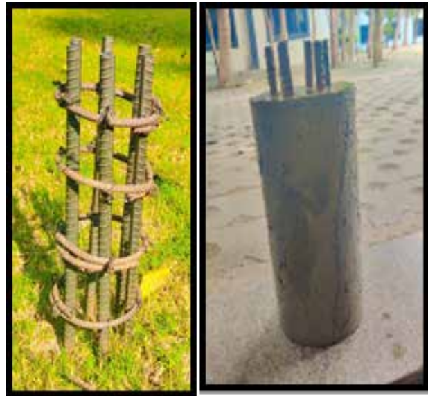
Fig 1: Tied reinforcement of column specimen & Column specimen after casting
